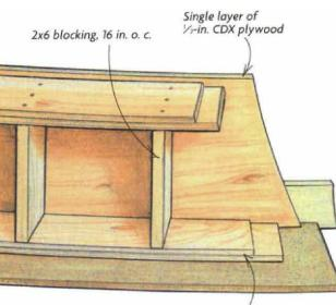
Bottom plate (two layers of 1/4-in. CDX plywood)
